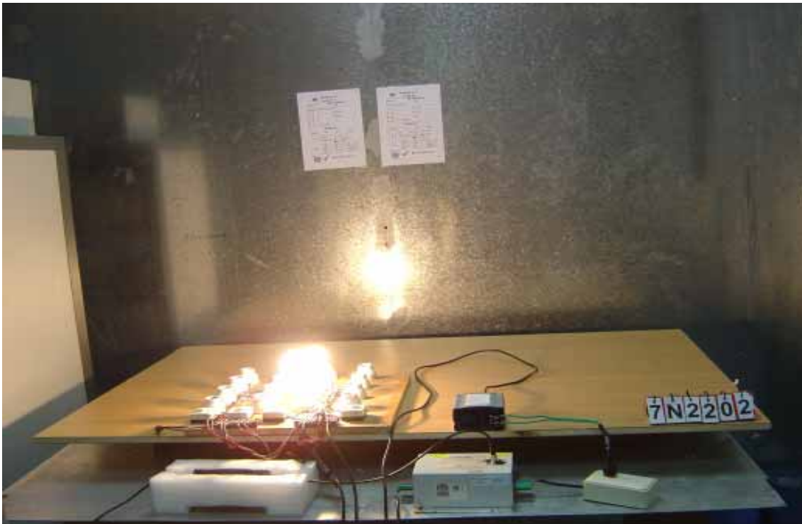
CS CONDUCTED DISTURBANCE IMMUNITY TEST
